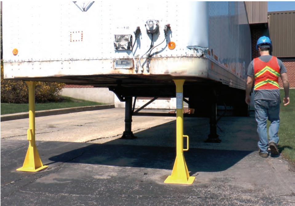
**ALWAYS use two jacks at the front of each trailer for good stability.** A single jack in the centre will not prevent side-tipping. If one or both of the legs give way, a single jack in front will act as a fulcrum and not be able to overcome the tipping action. Trailer must be secured with dock lock or wheel locks.
