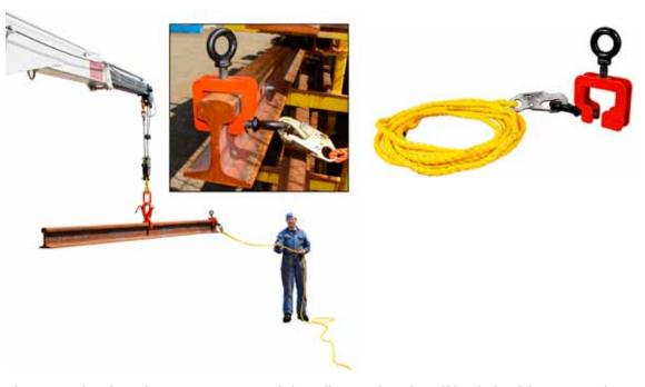
The IPS Rail Tether Clamp is a unique tool that allows rails to be off-loaded safely. Designed to attach quickly to the end of a rail, the tether clamp allows a worker to guide and control a rail during loading and unloading, and minimises the risk of accidental employee injury and property damage. Rope and attachment clasp included.
