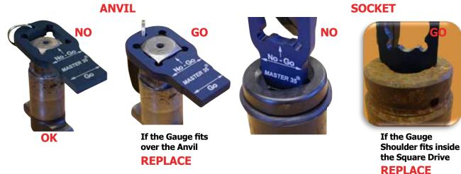
The Gauge is supplied with a Clip so it can be attached to a Key Ring or Belt to reduce the chances of it being lost.
