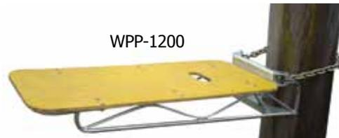
Standing platform is 1060 x 460mm with anti-slip surface. High tensile chain is supplied to suit wooden power poles up to 750mm in diameter. Tested and certified to working load limit 150kg. Frame work is zinc plated.
