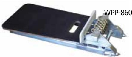
Made from steel and marine ply, finished with zinc plating. This unit is rated to a working load limit of 150kg. Standing platform measures 350 x 650mm, 3mm rubber is adhered for insulation and anti-slip properties. Will suit wooden power poles up to 400mm in diameter.
