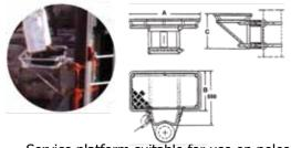
Service platform suitable for use on poles for maintenance of overhead equipment. Made of aluminium alloy, with double nylon straps and ratchet for pole attachment.
