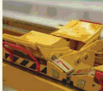
Hydraulic telescopic extended arm for bundle insertion
