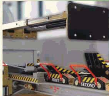
Hydraulic telescopic extended arm for bundle insertion
