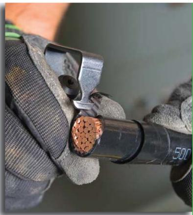
Capacity: THHN Cable Size Range: 10-625 mm2 Overall Cable Diameter: 4.5-40.0 mm
