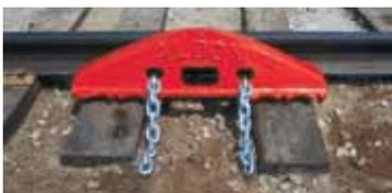
Cast in high strength alloy steel, these double-end rerailers can carry the weight of a 408 tonne (450 ton) rail car or locomotive. Rerailers are used in pairs but sold separately, both an inside and an outside rerailer is required per set (note that photos only illustrate OUTSIDE model). Chains which are sold separately secure the rerails to the rail, two are required per rerailer (so four are required per set).
