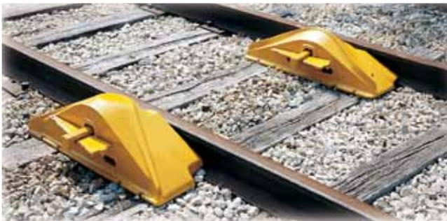
Double-ended "Burlington-Style" rerailers are locked to the rails by clamps and wedges and will not slip or kick out during rerailing. One **Inside** and one **Outside** make a pair. Rerailers are reversed in direction and exchanged in position to suit different derailed wheel situations. For use with standard size cars. **Used in pairs but sold separately: one inside rerailer and one outside rerailer.**
