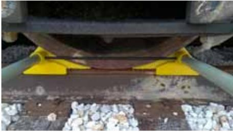
SPARK-PROOF Urethane Wheel Chocks are tough enough to block a tank car, but resilient enough that the car can be pulled over the chock by a locomotive without derailling. For chocking tank cars and other freight cars, loading or unloading hazardous materials and used where a spark from a steel wheel chock could ignite dust or fumes.
