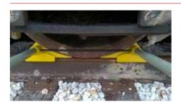
SPARK-PROOF Urethane Wheel Chocks are tough enough to block a tank car, but resilient enough that the car can be pulled over the chock by a locomotive without derailing. For chocking tank cars and other freight cars, loading or unloading hazardous materials and used where a spark from a steel wheel chock could ignite dust or fumes.
