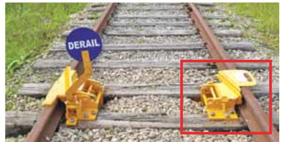
**NEVER use a SideKick alone. It should always be used in conjunction with the Aldon hinged derail model specified at the right. Workers must ensure that the derail and the SideKick are both in the same position (on or off the rail) at all times.**
