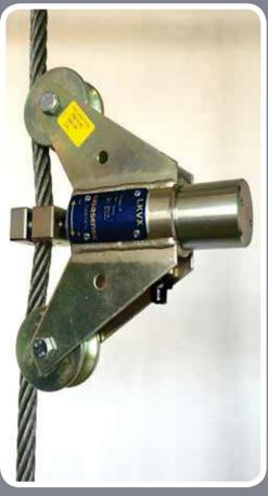
The LKVX Overload Guard is designed for use in potentially explosive atmospheres.
