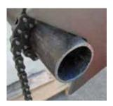
Cuts many materials including cast iron pipe, PVC pipe, and H-shaped steel.
