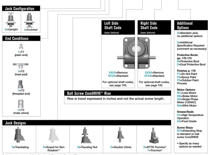
\*Standard trunnion mounts available on 2-ton through 20-ton jacks. (See page 173) \*\*Keyed for non-rotation is not a standard option. Contact Joyce/Dayton.
