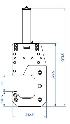
Hydraulically operated soft and fibre line cutting tool Lightweight aluminium and stainless steel construction Diver or ROV operable design Quick and efficient operation Long blade life ensures that tool maintenance
