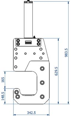
Hydraulically operated soft and fibre line cutting tool
