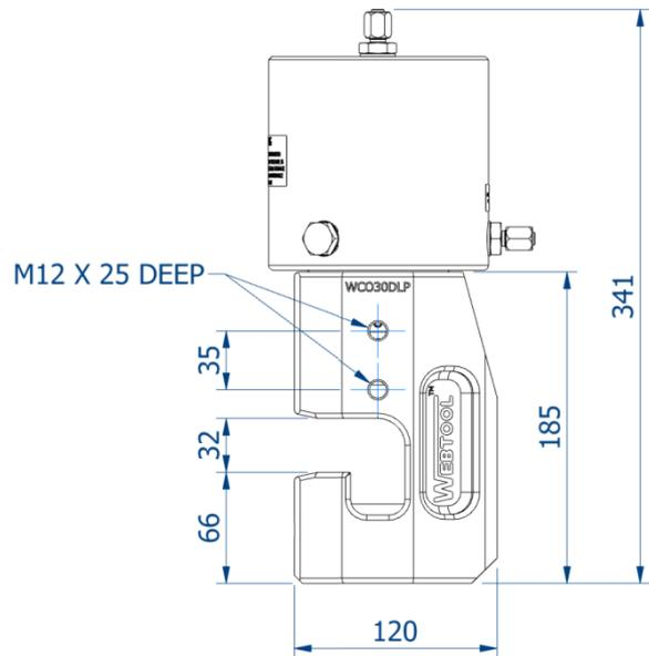
Heavy duty wire rope cutter designed for use in severe working conditions
