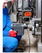
Image above: alkitronic® RCL pneumatic torque multiplier in operation on a plate heat exchanger. Image below: alkitronic® CLV-R
