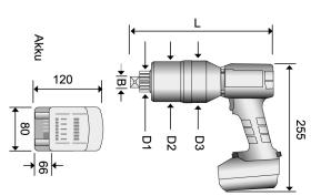
2 lithium-ion battery packs 18 V, 5.2 Ah, battery charger, tool case supplied as standard Repeat shut-off accuracy ± 3% (same bolting connection). All alkitronic® torque multipliers are CE-certified.
