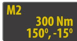
Torque/angle procedure for high-quality bolting connections. Display example of pre-torque, angle and loosening angle.
