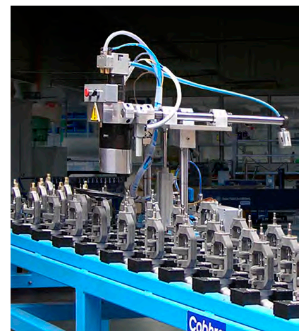
alkitronic® CLV operating in a preassembly and final assembly workstation. Remote controlled continuous tightening in semiautomatic operation.
