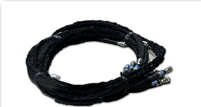
HIGH PRESSURE HYDRAULIC CIRCUIT HOISING RATED TO 700 BAR WITH INTEGRATED BURST PROOF SLEEVING, COUPLINGS, HYDRAULIC CIRCUIT IDENTIFICATION
