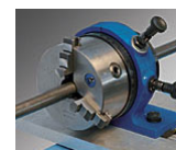
Mechanical spindle for the bending plan regulation.
