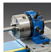
The 2 interchangeable outlet shafts of the standard equipment.
