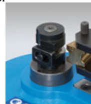
Reduced shaft for bending with radii less than 30 mm.
