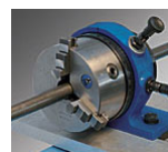
Mechanical spindle for the bending plan regulation.
