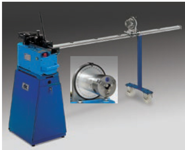
Electric UNI 60 A, version with moving plane of bend and universal base.
