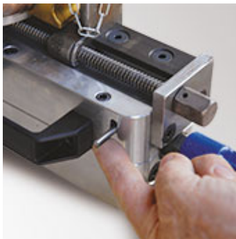
Anti-rotation and return device of the wind lever.
