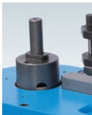
Provided reduced shaft to use with special formers and guides for bending radii which are less than 30 mm.
