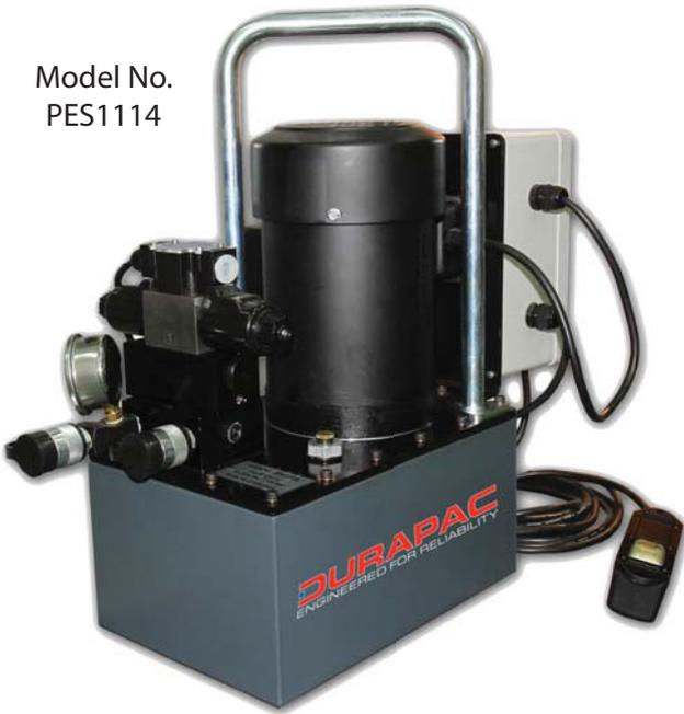
Cool Running & Dependable Performance High first stage performance is achieved through field proven Gear Pump technology. In addition to gear pumps, an unloading valve passes full power to the second stage once crossover pressure is reached. No power is lost and less heat is generated.
