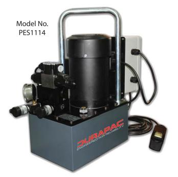
Cool Running & Dependable Performance High first stage performance is achieved through field proven Gear Pump technology. In adition to gear pumps, an unloading valve passes full power to the second stage once crossover pressure is reached. No power is lost and less heat is generated.
