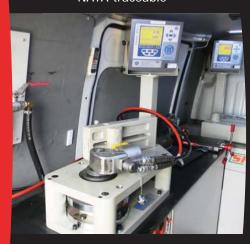
**NOTES:** Mine spec Requires 230VAC external power source. External air supply required for pneumatic tools
