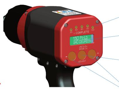
5 yellow LEDs indicate percent of set torque achieved. All LEDs turn green when set torque is reached and red if the set torque is not achieved.
