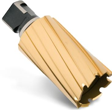
These special Twister Bits™ have a 50mm (2") depth of cut and are specifically design for Crane & Girder Rail applications. "TiN" coated (Titanium Aluminium Nitride) for extended tool life and Twister Bit™ shank. \* Twister bits can only be sharpened by specialists, contact your nearest SF branch for more details.
