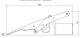
Wedge with Hydraulic Cylinder = 8.5 kgGross Weight = 9.8 kg
