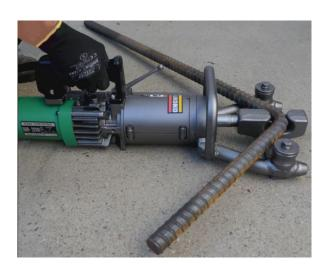
Double Acting Hydraulic Cylinder Capable of Bending or Straightening up to 32mm Rebar.
