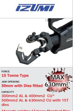
\*Accepts existing 12 tonne Standard Dies Nest/Indent & "C" connector Dies when used with 15T-PU-ADAPTOR
