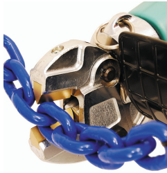
Cutting Hoist Chain
