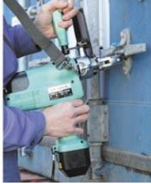
Cutting Container Seal
