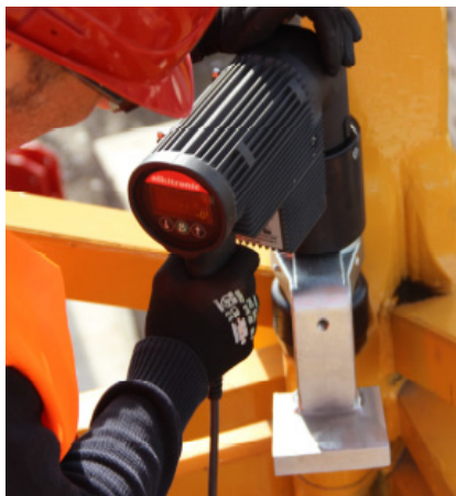
Crane assembly using angled electric torque multiplier EC-A, EF-A with special support for Liebherr
