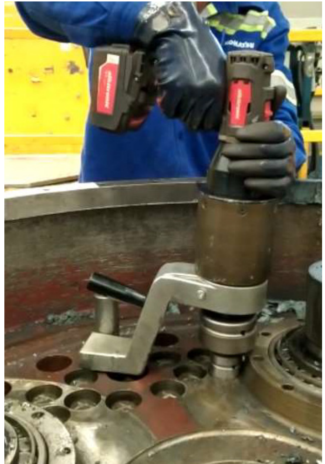
Komatsu - Mining truck 793E - Upper inner coupling Torque: 1918 ft.lbs/2,600 Nm Tools used: EAF 2/600
