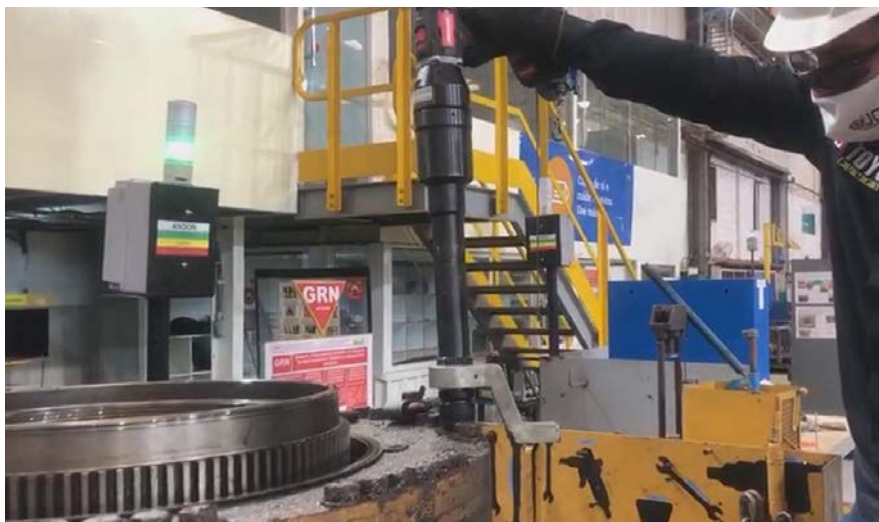
Vale Caue Mine - Mining truck CAT 793D – Brakes Torque: 369 ft.lbs/500 Nm Tool used: EAF 2/280 N12
