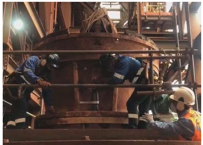
Vale 511D Mine - Sandvik Cone Crusher CS 660 Torque: 2323 ft.lbs/3,150 Nm Tool used: EAF 2/600
