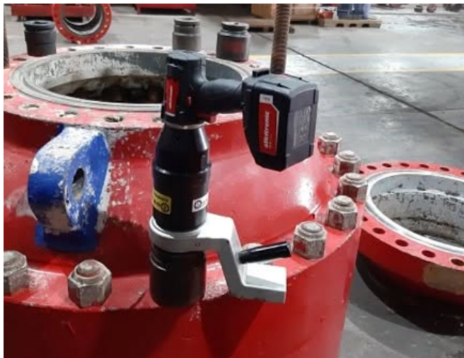
Working on sealing a large valve, which is used to control wellbore fluids with an EAF. Torque: 3600 Nm.
