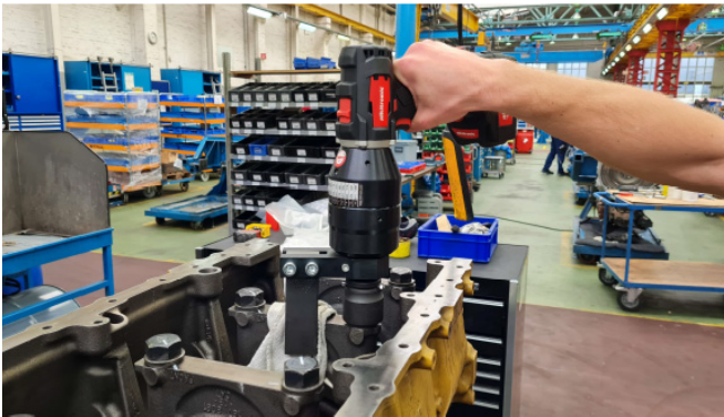
Tightening the main bolts (crankshaft bearings) of a Caterpillar C18 engine using EAF 150 with special support. (Here without crankshaft for testing.)
