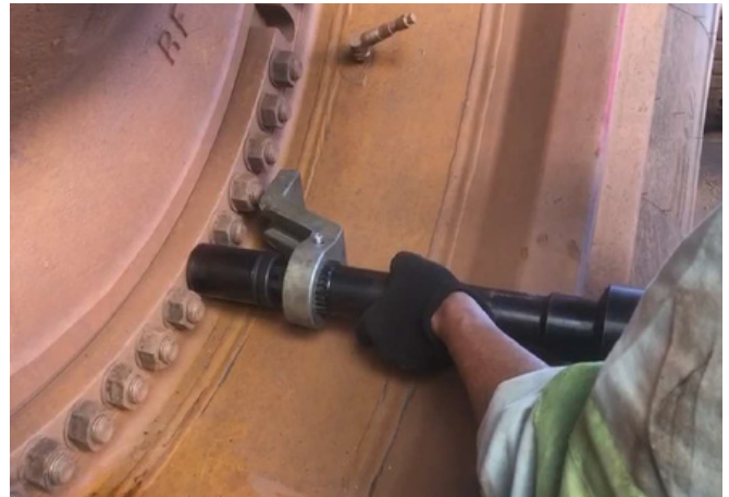
EAF 2/280 N12 on a mining truck Komatsu 730E Wheel Torque: 1,850 Nm
