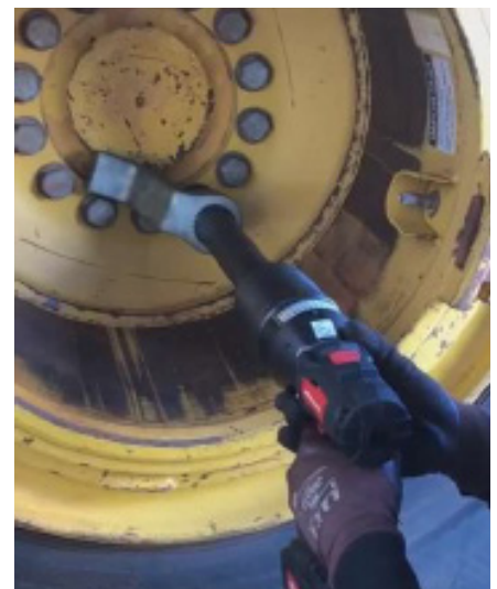
EAF 2/280 N12 on a Wheel Loader John Deere 744K-II – Wheel – Torque: 1,000 Nm
