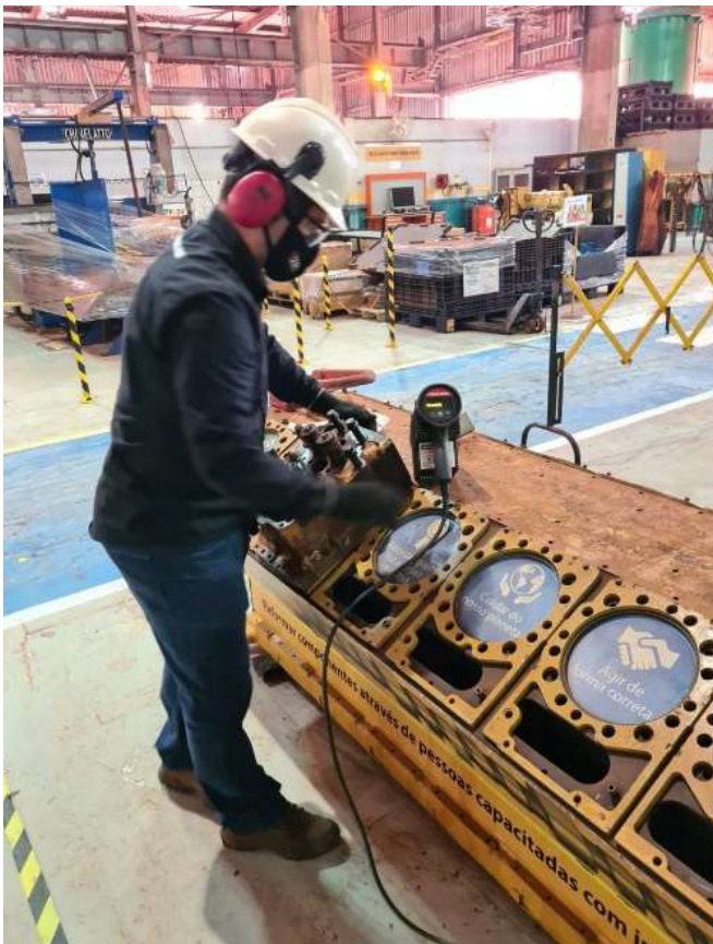
Vale N5 Mine – CAT Engine head Torque/rotation angle: 258 ft.lbs/350 Nm + 90° Tools used: EC-S 65
