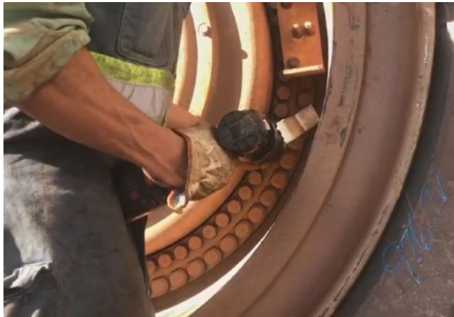
EAF 2/280 N12 on a mining truck CAT 793D Wheel Torque: 1,000 Nm
