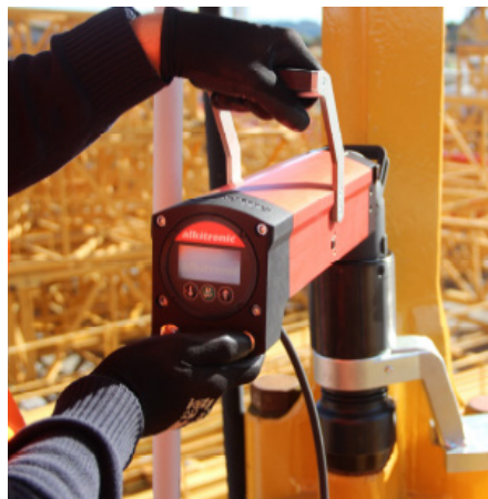
Crane assembly using angled electric torque multiplier EC-A, EF-A with special support for Liebherr
