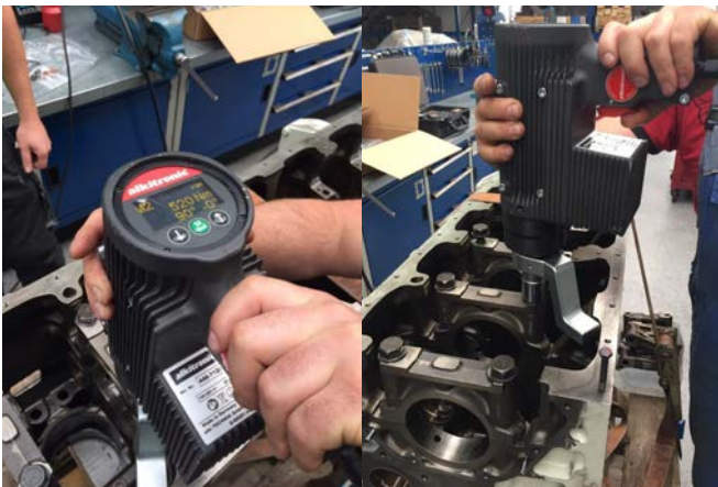
Connecting rod bearing assembly on a MAN engine EAF 150 (Pre-torque and angle of rotation)
