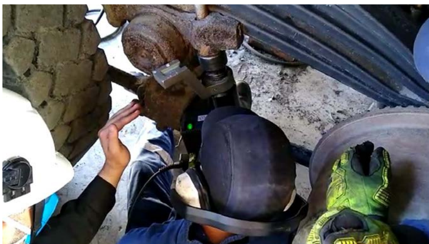
Mosaic Fertilizers - Scania truck G440 – Spring bar Torque: 1254 ft.lbs/1,700 Nm Tool used: EC-S 60
