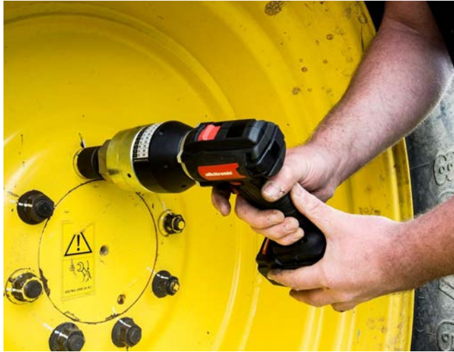
Rim exchange of a forage harvester using EAF – torque: 550 Nm
