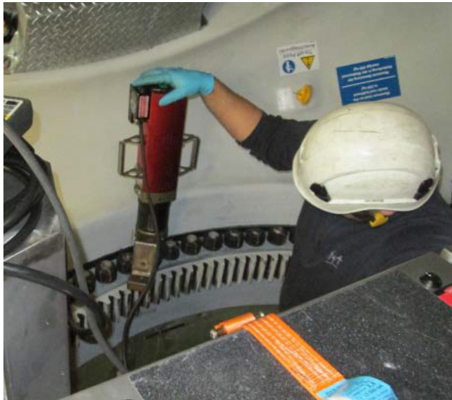
The alkitronic EF in use at the rotor blade bolting.
