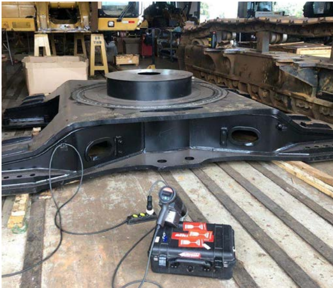
Sotreq Caterpillar - Tracked excavator CAT 744KII – Turntable Torque/rotation angle: 332 ft.lbs/450 Nm + 90° Tools used: EC-S 65, EAF 2/600
