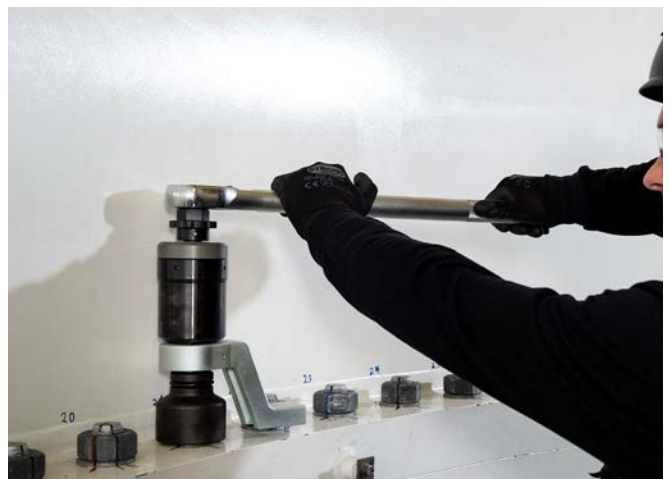
EC-S 65 M36-HV Maintenance on a tower bolt, torque: 2,795 Nm
