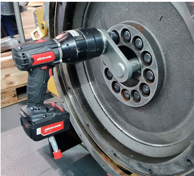
Bolting a flywheel to a Caterpillar 12-cylinder engine using EAF 150 with special support arm
