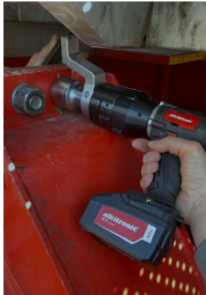
Dis-/Assembly of fairground ride: 800 to 1,225 Nm with different bolt sizes, limited space (40mm) alkitronic® tools used: EAF 2/150, XCE Link 3:1 AF 46
