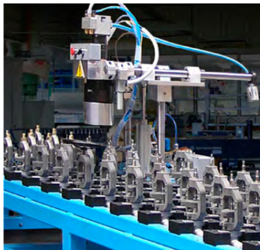
Alkitronic PV-F operating in a preassembly and final assembly workstation. Remote controlled continuous tightening in semi-automatic operation.
