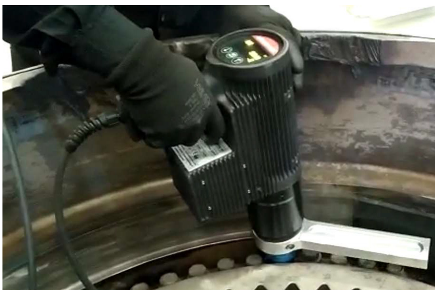
Komatsu - Mining truck 730E - Bearing lower coupling Torque: 996 ft.lbs/1,350 Nm Tool used: EC-S 60
