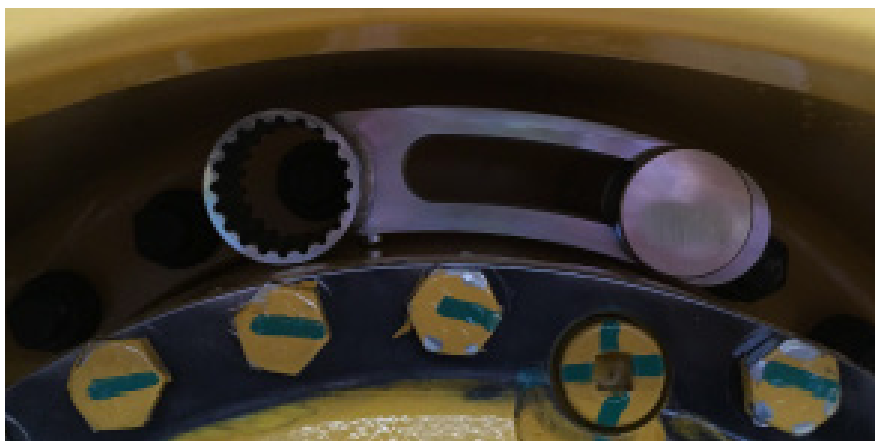
Curved sliding special support arm for use on a wheel rim for Bell Equipment
