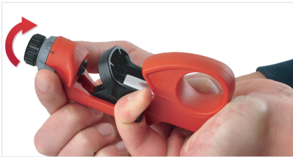
Unlock the cable stripper by turning the adjusting ring to the round-cut symbol (⊙)
