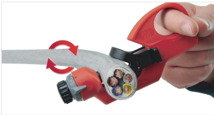
Place the tool on the marking of the stripping length and make the round cut
