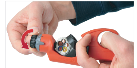
Regulate the cutting depth by turning the adjustment knob (clockwise)
