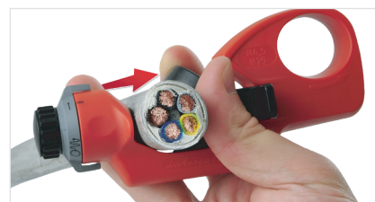
Shift the adjusting ring to the spiral-cut symbol (⊙) to fulfil the working process
