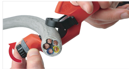
Shift the adjusting ring to the spiral-cut symbol (⊙) to fulfil the working process
