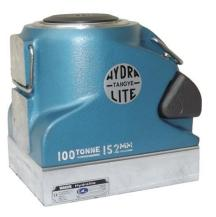
The 100 tonne Hydralite is powered by two internal pumps. The low pressure, fast-speed plunger moves the ram out quickly, up to a load of about 8 tonnes on the ram, before transfer to the high pressure plunger becomes necessary. The lift of ram per stroke of lever is 1.1mm on low pressure and 0.1mm on high pressure.
