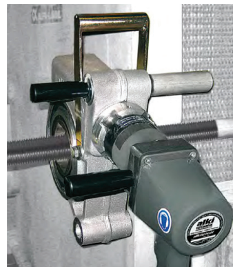
Image above: alkitronic® RCL pneumatic torque multiplier in operation on a plate heat exchanger. Image below: alkitronic® CLV-R
