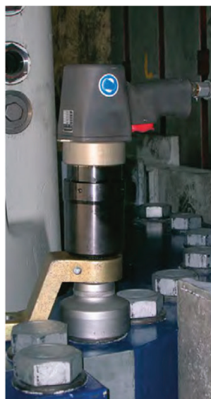
alkitronic® CLD torque multipliers in use (figures on the right). Screw connections at a bolt circle and a diesel unit for large construction machines
