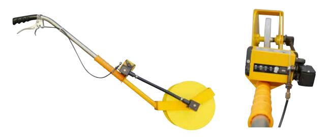
For accurate measuring of rail track. This robust, quality measurer was designed with input from international railroad companies and is in daily use worldwide. The heavy duty measuring wheel incorporates metal side plates keeping the wheel stable on the rail.
