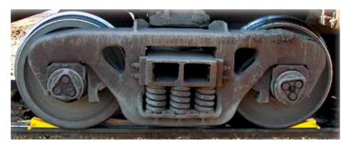
Wooden wedges can only be run over once and they can litter the track with splinters. A car can be pushed over the NINE LIVES wheel wedge.
