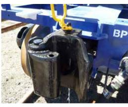
Coal locos and wagons complete with Bradken couplings and yokes with Miner Crown SE draft gear.
