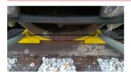
SPARK-PROOF Urethane Wheel Chocks are tough enough to block a tank car, but resilient enough that the car can be pulled over the chock by a locomotive without derailing. For chocking tank cars and other freight cars, loading or unloading hazardous materials and used where a spark from a steel wheel chock could ignite dust or fumes.
