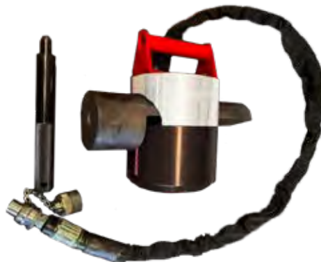
Assembled JIG c/w DURAPAC RG-502/RT 50Ton Cylinder
