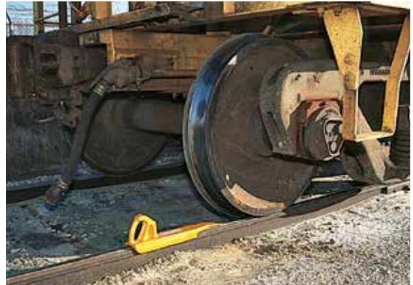
Replace skids when tongues become deformed. Skid tongue must lie dead flat on the rail to be effective.
