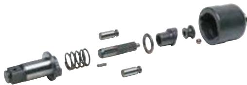
The pin-clutch system produces a single impact for each cycle. The strokes are made by two pins which are pitched directly on the shaft. This creates a balanced impulse and a lower vibration level compared to the others systems.
