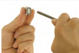
2. Thread Wire through Oval Sleeve
