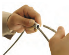
3. Loop the Wire Rope from Eyelet
