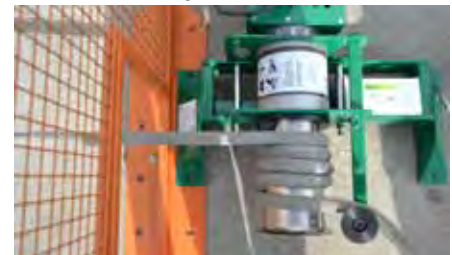
Designed for Greenlee winch Floor Mount (00865)
