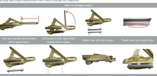
Place liners in jaw, stubs on liners will fit into holes in jaw frames.
