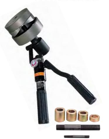
Our mild steel punches have 3 cutting crown edges and require less force to pull through than 4 crown punches
