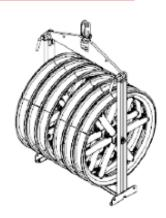
Six sheave running out block suitable for six bundled conductors, using 2 pilot ropes. Aluminium sheaves mounted on sealed ball bearings. Grooves lined with nylon. Steel frame with non-fleeting devices on lateral sheaves. Demountable attachment revolving at 90°.
