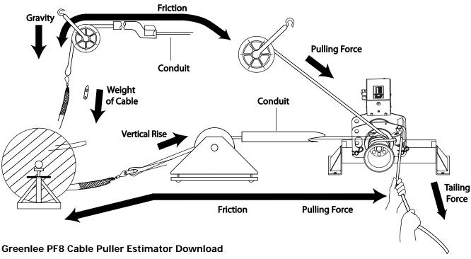
To give an approximation of the pull force that will be required to install electrical cable into a conduit, there are many unknown factors involved that prohibit giving exact results. Most notable amongst these is the coefficient of friction, occupancy of conduits (existing cables), lubrication, surface texture, and lay of the cable are never uniform along the length of a conduit run.
