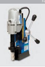
Large 38mm x 50mm capacity. Uses Mag Drill Annular Cutters. Positive slug ejection. Durable and powerful magnet. Wide range of accessories are available. Feed handles quickly change from side to side. Lift detector safety system with rear mounted controls. Gravity fed coolant system. Carrying case included with one year warranty.
