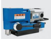
Ultra Low Profile lightweight right angle drill with large capacity. Patented quill feed arbor for smooth cuts and minimal maintenance. Uses RotaLoc Plus™ annular cutters which requires no tools for installation or removal. Pilot light; positive slug ejection; high torque gearing and lift detector safety system. Feed handle switches easily from side to side. Ratchet can be used in place of feed handle. Rear mounted controls. Carrying handle. Carrying Case included. Two year warranty.
