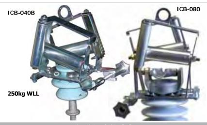
Insulator cable bracket to suit vertical post insulator with top clamp. The unit folds together on a hinge and has a hand screw up handle. A top ring allows the unit to be carried easily or lowered from pole tops with rope. The ICB-040B sits close to the top of the insulator where the ICB-080 is raised up higher.
