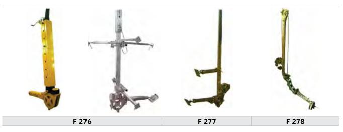
Telescopic rods for laying underground cables and pulling wire rope inside the pits. Mounted on pullers properly arranged, they permit to pull the wire rope inside the manholes. Made with galvanised/painted steel, the rods are easily demountable to facilitate the transport. Guide system with 360° swivelling pulley.
