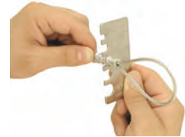
QUALITY CHECK SLEEVE WITH GAUGE, PASS THROUGH SWAGING COMPLETE!
