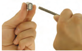
2. Thread Wire through Oval Sleeve
