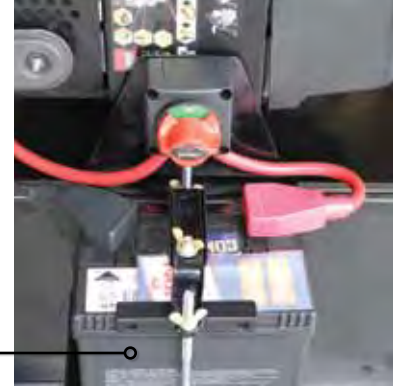
12 V BATTERY with isolation switch
