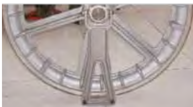
"-S" Traveller Stand mounted to the bottom of roller
