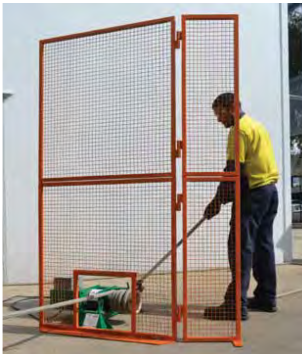
Designed for Greenlee winch Floor Mount (00865)
