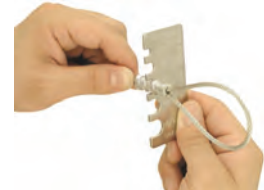
QUALITY CHECK SLEEVE WITH GAUGE, PASS THROUGH SWAGING COMPLETE!
