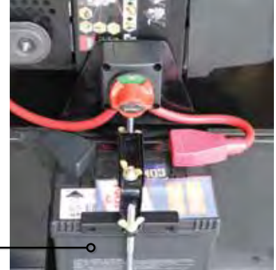
12 V BATTERY with isolation switch
