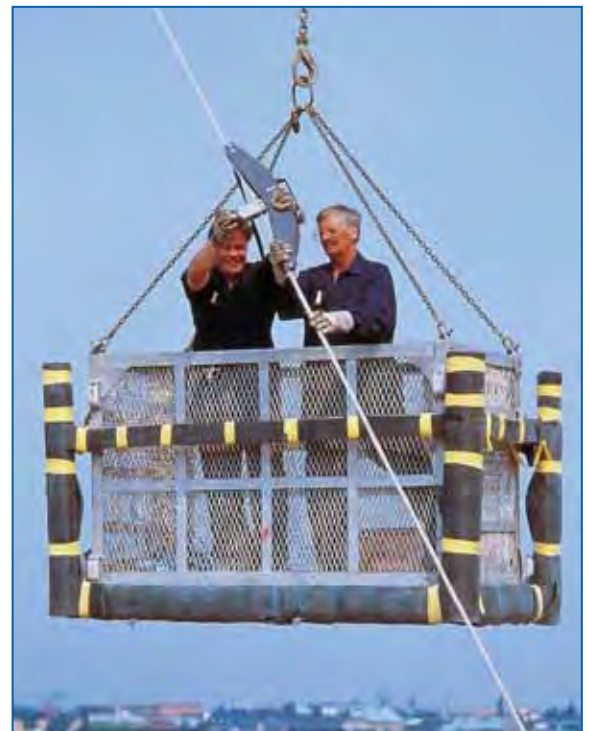
Also when stay ropes are difficult to reach the lightweight RTM 20D is easy to handle. The picture shows control of tension from a crane operated working platform.
