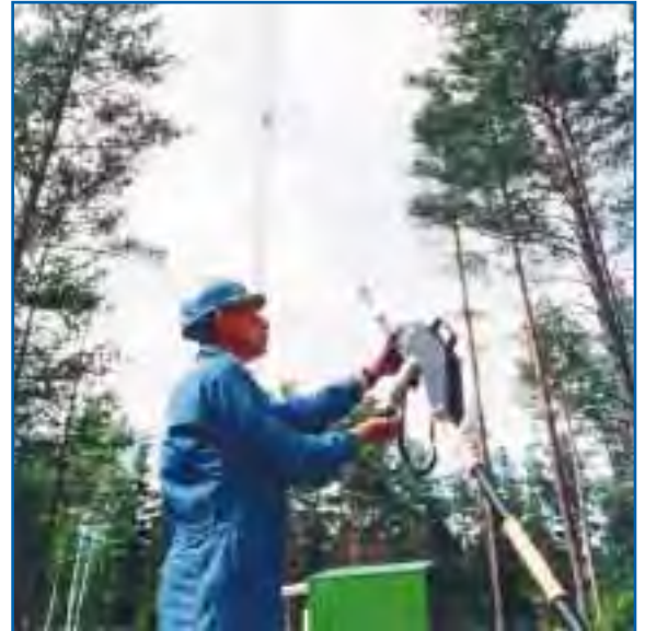
The rapid growth of mobile telephones all over the world need a lot of transmission masts. For accurate operation the masts have to be guyed in a stable position, unaffected by strong winds. Control of tension in the various supporting stay ropes is easily made by using PIAB RTM 20D.
