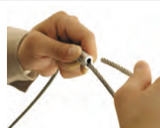
3. Loop the Wire Rope from Eyelet
