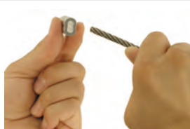
2. Thread Wire through Oval Sleeve
